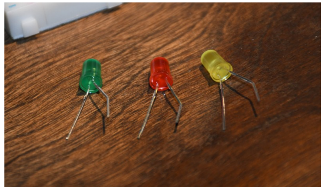
Figure 14: The three LEDs. Green for ready. Red for alarm. Yellow for silence.
