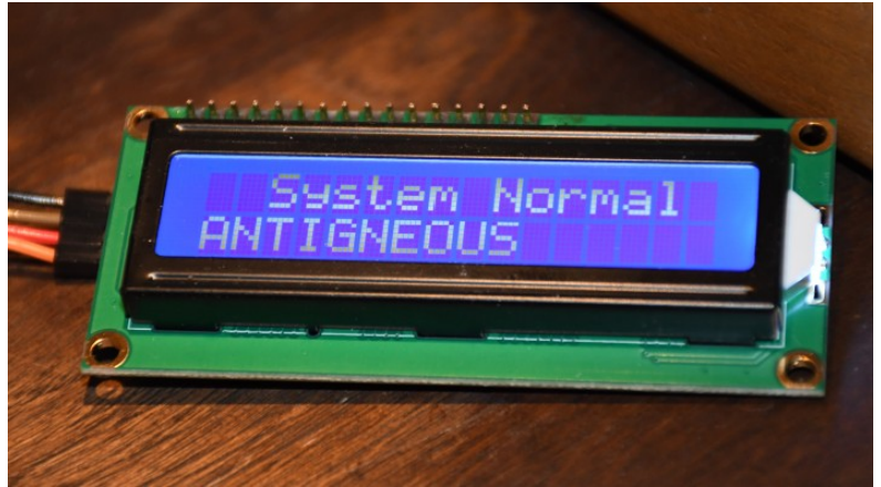
Figure 9: Successful bootup of the ESP-32. This will most likely NOT be what you see, as this board has already had Antigneous installed on it once, and is able to pull from stored settings, which won't likely be present on your board.
