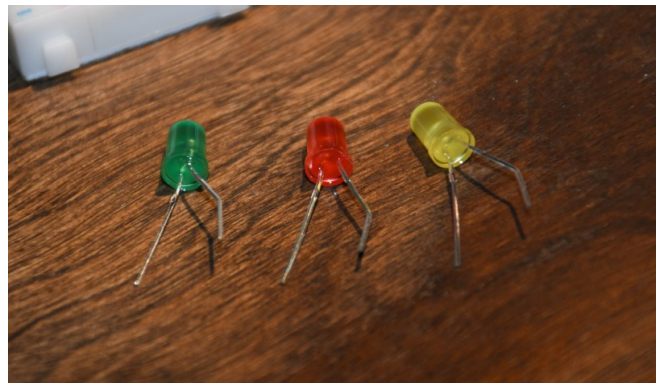
Figure 13: The three LEDs. Green for ready. Red for alarm. Yellow for silence.
